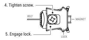
BOTTOM VIEW SHOWING CORRECT INSTALLATION
